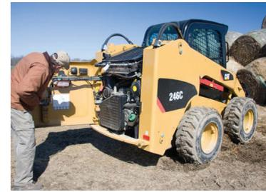
These inspections only take a few minutes and they are one of the best ways to detect small problems before they become serious. Follow walk around guidelines in the OMMs, which should be kept on machines. Supervisors must allow time for a thorough evaluation. Start by making
