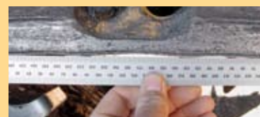
Shown above, a SystemOne link assembly with conventional idler and the scalloping that resulted from its contact with the link rail.
