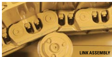
Shown above, a SystemOne link assembly with conventional idler and the scalloping that resulted from its contact with the link rail.
