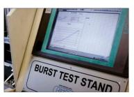
Cat hose is burst tested by applying pressure at a constant rate until it reaches a burst pressure of four times the normal operating pressure.
