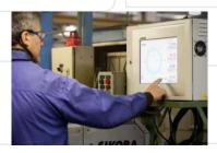
Cat hose is carefully monitored to ensure precise inner and outer diameter measurements are maintained. This provides precise coupling retention capability.
