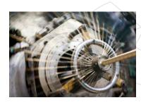
Before application, the hose is routed through a cooling chamber until it reaches a suitable temperature. This prevents perforation of the hose as the high tensile strength reinforcement wire is applied.
