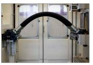
To simulate punishing conditions, Caterpillar impulse-tests hose assemblies at 130% of operating pressure for one million cycles—double the SAE standard of 500,000 cycles.
